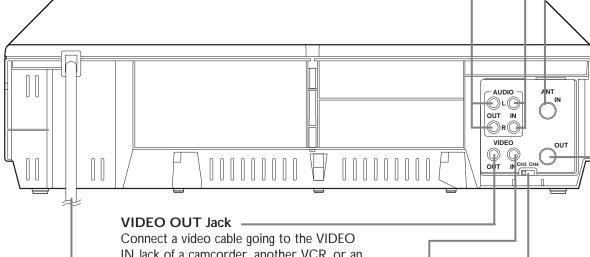
Connect a video cable going to the VIDEO IN Jack of a camcorder, another VCR, or an audio-visual system (monitor, laser disc player, digital video disc player, etc.) here. Details are on pages 34 and 40.
